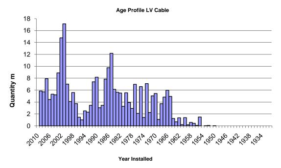
The cable installation rate shows a strong correlation with reduction in overhead line installation.
