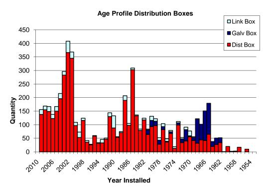
Replacement of the older galvanised boxes is underway as overall deteriation is identified during inspection.
